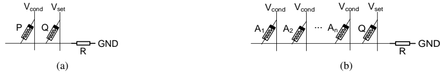
Figure B1 The IMPLY gates. (a) The original IMPLY gate [7]; (b) The n-input IMPLY gate [22].
