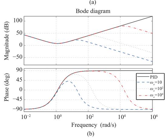
**Figure 1** (Color online) Frequency analysis of the feedback compensator of second-order LADRC. (a) Block diagram of second-order LADRC; (b) Bode plots of  $C(s)$  and  $C_{PID}(s)$ , in which  $K_c = 2.5$ ,  $\tau_I = 1.777$ ,  $\tau_D = 0.4$ .
