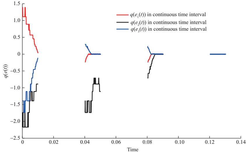
**Figure 2** (Color online) Trajectory of  $q(e(t))$  in continuous time interval under quantizer (7) with initial condition  $q(e(0))$ .
