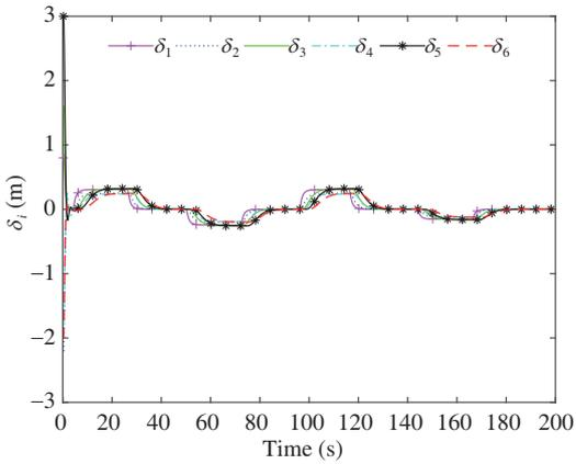
**Figure 7** (Color online) Desired spacing errors of vehicles in different initial states.
