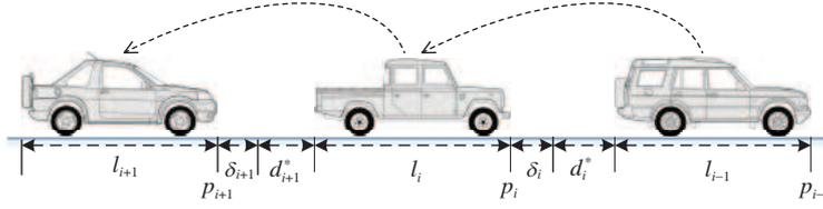
**Figure 1** (Color online) A schematic of the vehicle CACC platoon system.
