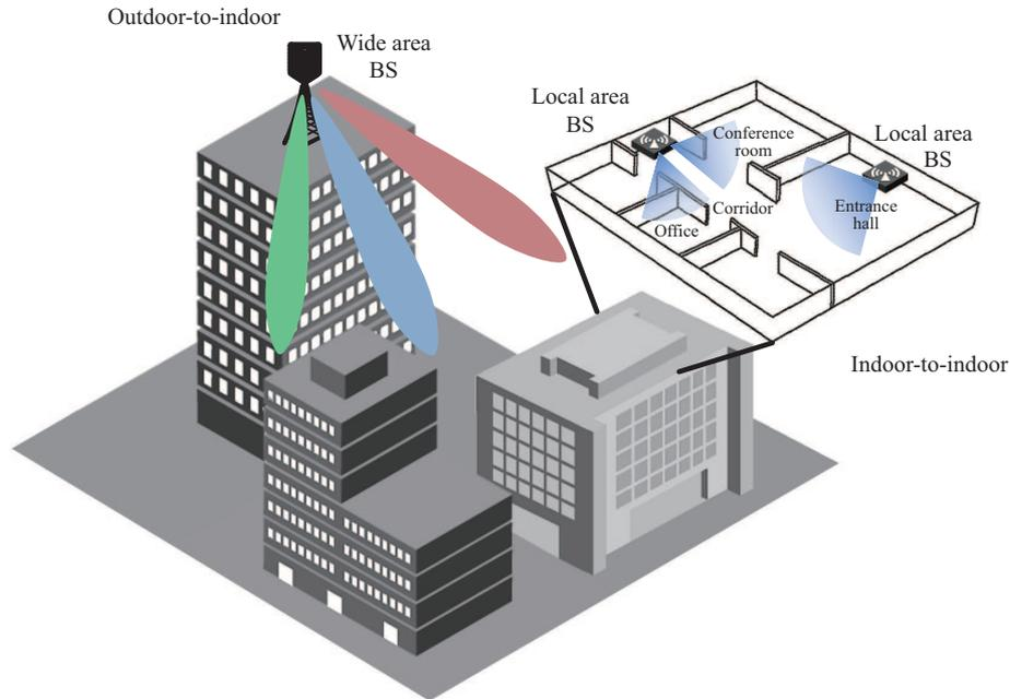
**Figure 1** (Color online) Illustration of a potential mmWave indoor and outdoor cooperative cellular network for in-building coverage, including a highly directional beam in outdoor-to-indoor channels and a wide beam in indoor-to-indoor channels.
