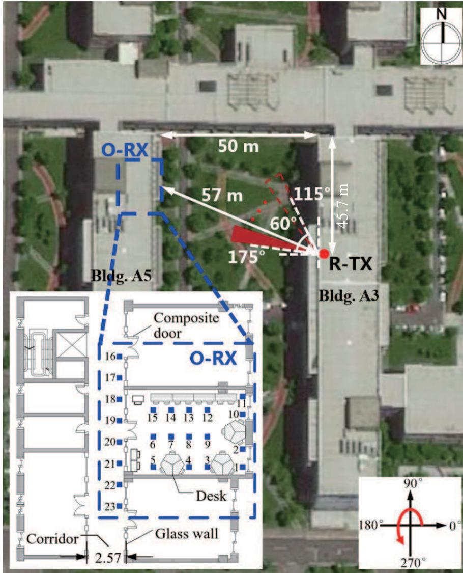
**Figure 2** (Color online) General plan view of O2I scenario. The TX is mounted on the rooftop of Building A3, and indoor RXs are located on the third floor of Building A5, which are all in the illuminated area.
