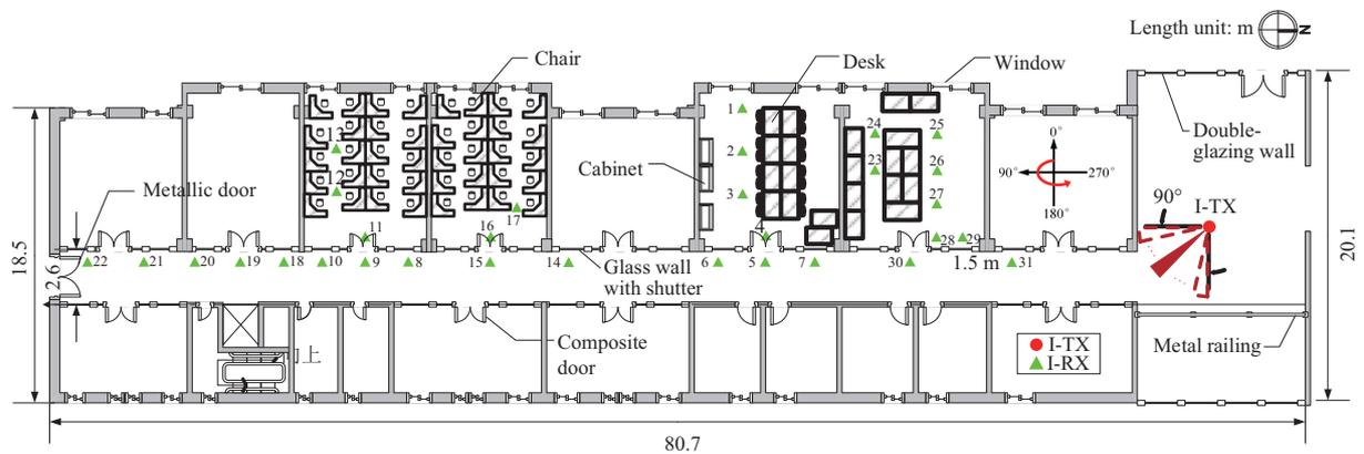
**Figure 3** (Color online) Layout of indoor TX and RX locations, where the red dots and green triangles represent the TX and RX locations for the indoor measurements, respectively.
