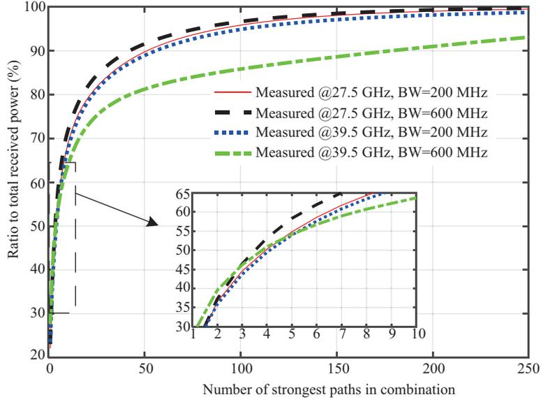
**Figure 9** (Color online) Power ratio of the combined directional beam to the total varying with the number of strongest paths in combination.
