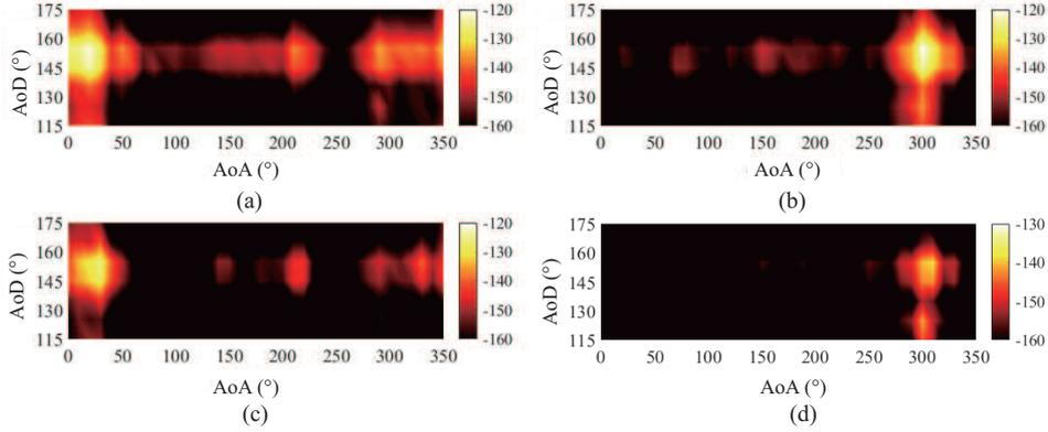
**Figure 8** (Color online) Double-directional path loss distributions in the AoA-AoD plane with sounding bandwidth of 200 MHz. (a) 27.5 GHz, O-RX 1; (b) 27.5 GHz, O-RX 2; (c) 39.5 GHz, O-RX 1; (d) 39.5 GHz, O-RX 2.
