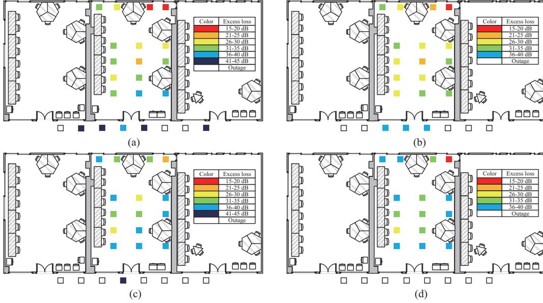
**Figure 7** (Color online) Excess losses relative to free space path losses for all O-RX locations. (a) and (b) at 27.5 GHz with bandwidths of 200 and 600 MHz, respectively, as well as (c) and (d) at 39.5 GHz.
