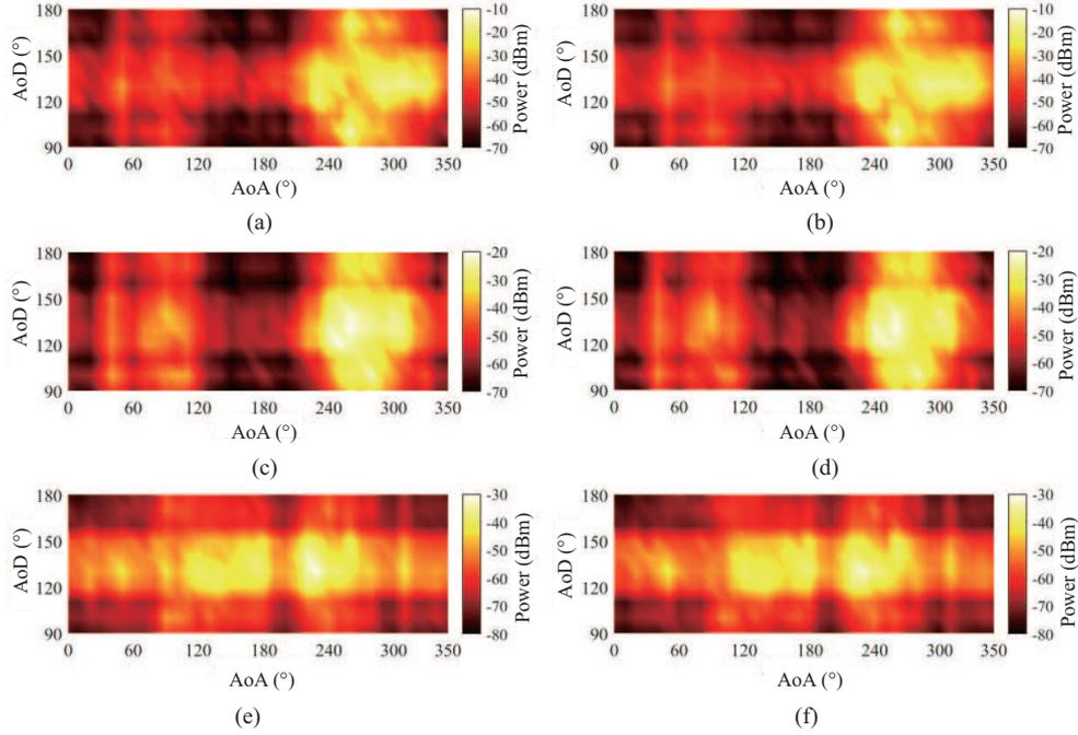
**Figure 6** (Color online) Double-directional APS at 27.5 GHz. (a) and (b) for RX 30 with bandwidths of 200 and 600 MHz, respectively, as well as (c) and (d) for RX 5 and (e) and (f) for RX 28.
