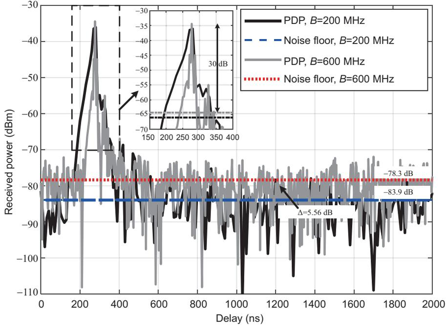
**Figure 4** (Color online) Comparison of the measured directional PDPs for I-RX 5 at 27.5 GHz with bandwidths of 200 (black line) and 600 MHz (gray line).
