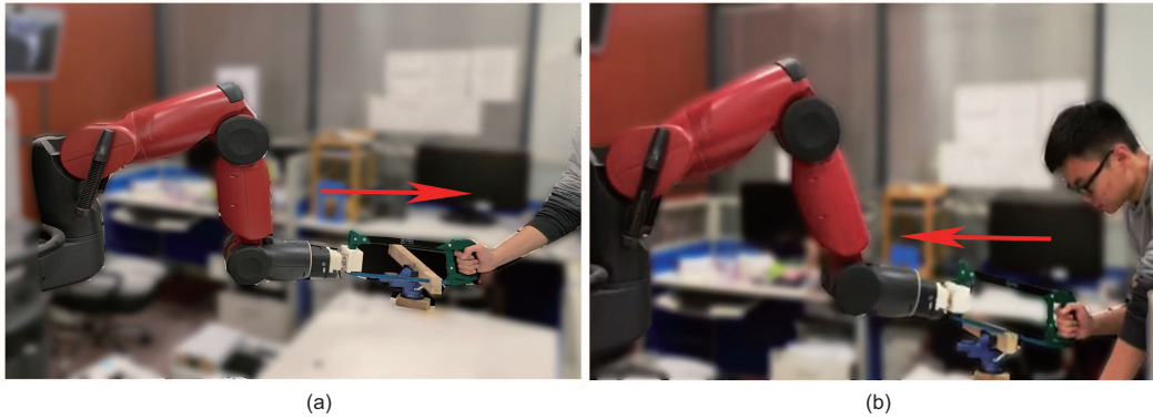
Figure 4 (Color online) The experimental set-up for the sawing task. (a) The human partner actively pulls the saw. The impedance of the robotic arm increases gradually from a small value to some extent. (b) The robot actively pulls the saw back owing to the large impedance. The human partner relaxes his muscle strength in this phase.
