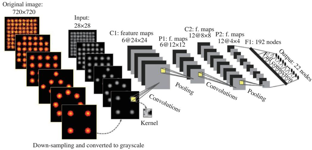
**Figure 5** (Color online) Schematic diagram of CNN-based constellation diagram analyzer for the OSNR estimation and modulation format identification [20].
