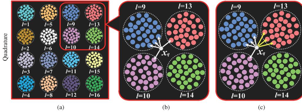
**Figure 4** (Color online) (a) 16QAM constellations with the corresponding labels; (b) KNN-based decoders when  $k$  is valued in 5; (c) DW-KNN-based decoders when  $k$  is 7 for the nonlinearity compensation [15] ©Copyright 2016 IEEE.
