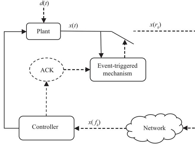
**Figure 1** Configuration of the event-triggered control with disturbances and transmission delays.
