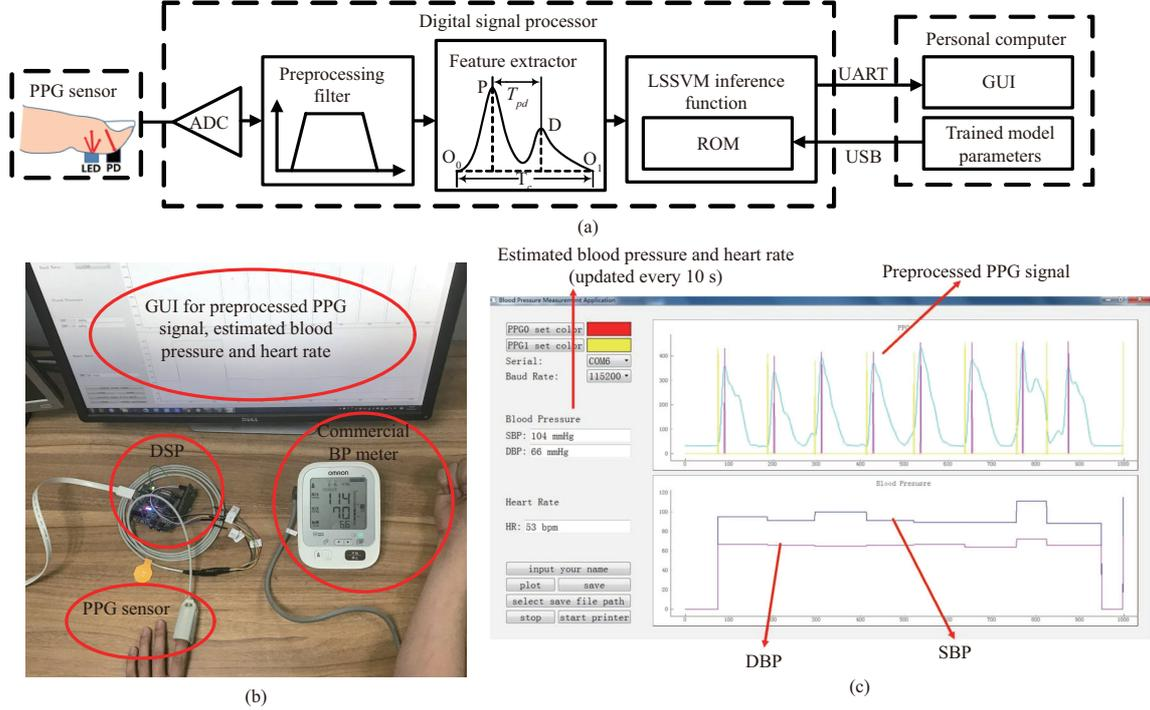
**Figure 1** (Color online) (a) Overall system architecture; (b) prototype for the proposed system; (c) GUI of the proposed system.
