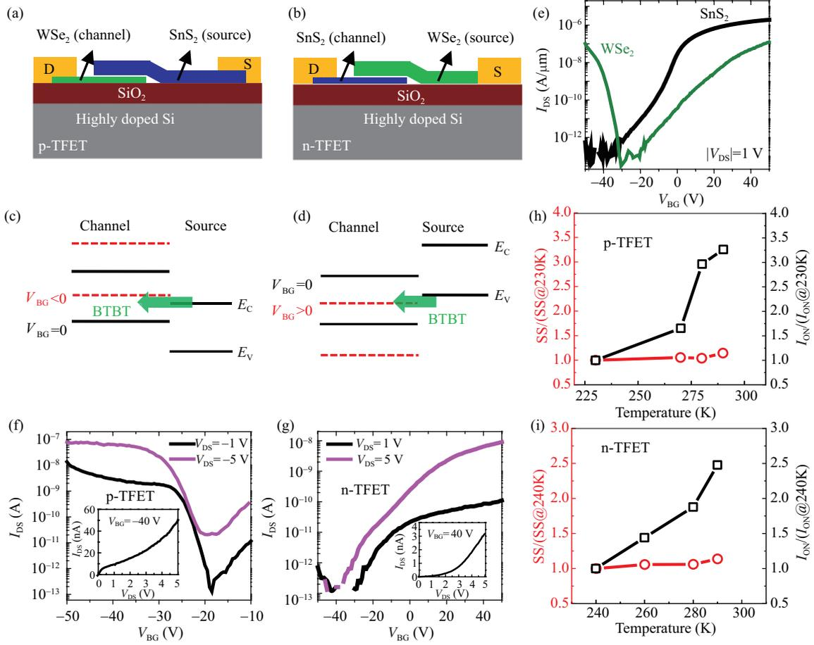
**Figure 1** (Color online) The schematic structures of p-TFET (a) and n-TFET (b). The band alignment of p-TFET (c) and n-TFET (d) in the off-state and on-state. The transfer characteristics of the WSe<sub>2</sub> and SnS<sub>2</sub> FET (e). The measured transfer characteristics of p-TFET (f) and n-TFET (g) at room temperature; (Inset) the corresponding output characteristics. Temperature-dependence characteristics of the p-TFET (h) and n-TFET (i).
