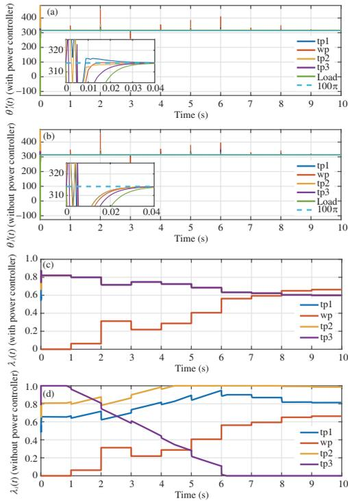
**Figure 1** (Color online) (a) and (b) Frequency trajectories of each node; (c) and (d) power output ratio.
