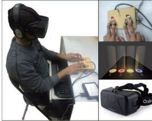
Figure 5 (Color online) Immersive visuo-haptic game comprising stimulus-response tasks using fingertip pressure control in a virtual reality environment.
