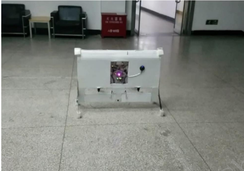
Indoor Hover Flight. (Only IMU and ultrasonic sensors are used for measurements)
