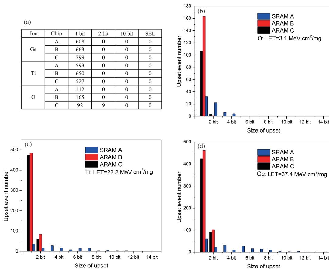
**Figure 1** (Color online) (a) Upset in logical word of SRAM in the experiments. The size of upset in physical address on three SRAMs in the experiments at O exposure (b), at Ti exposure (c), and at Ge exposure (d).
