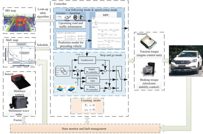
Figure 1 (Color online) Control architecture of the proposed longitudinal driving strategy.
