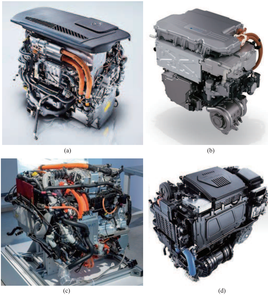
Figure 2 (Color online) Compact fuel cells developed by advanced automotive manufacturers. (a) Mercedes-Benz fuel cell; (b) Honda fuel cell; (c) BMW fuel cell; (d) Hyundai fuel cell.
