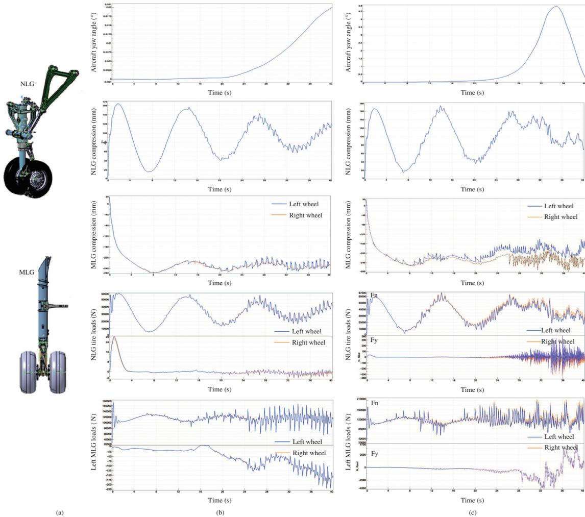
**Figure 1** (Color online) Taxiing stability simulation results. (a) Simulation model of NLG and MLG; (b) taxiing in symmetric scenario; (c) taxiing with lateral disturbance.
