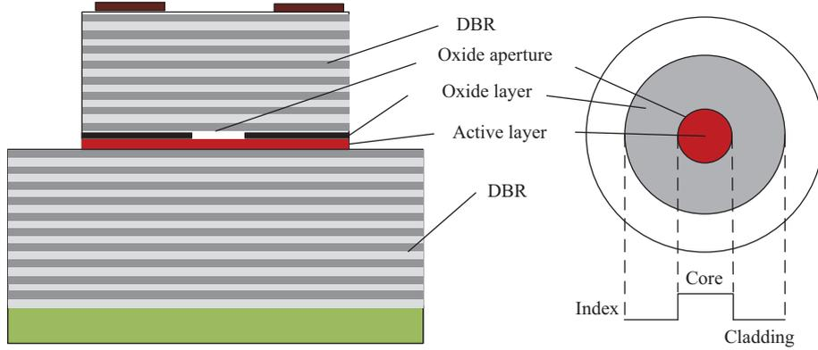
**Figure 1** (Color online) VCSEL structure and equivalent step-index optical waveguide.
