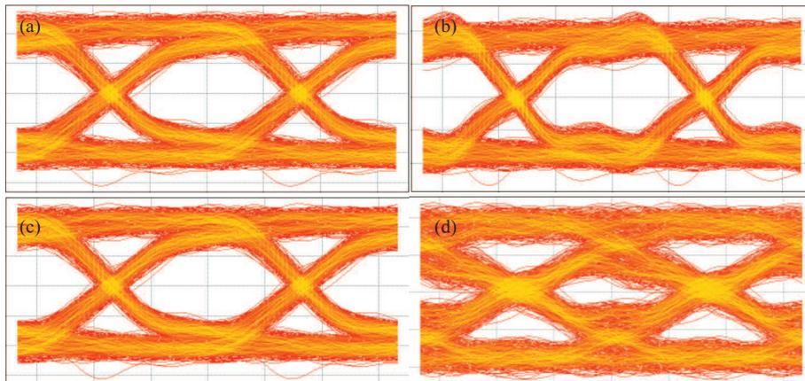
**Figure 5** (Color online) Eye diagram of (a) BTB and (b) 300 m propagation of VISTAS without our proposed method, (c) BTB and (d) 300 m propagation of VISTAS with our proposed method.
