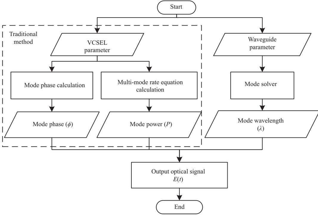
**Figure 2** Calculation flowchart of the output optical signal  $E(t)$  based on our proposed VCSEL model.
