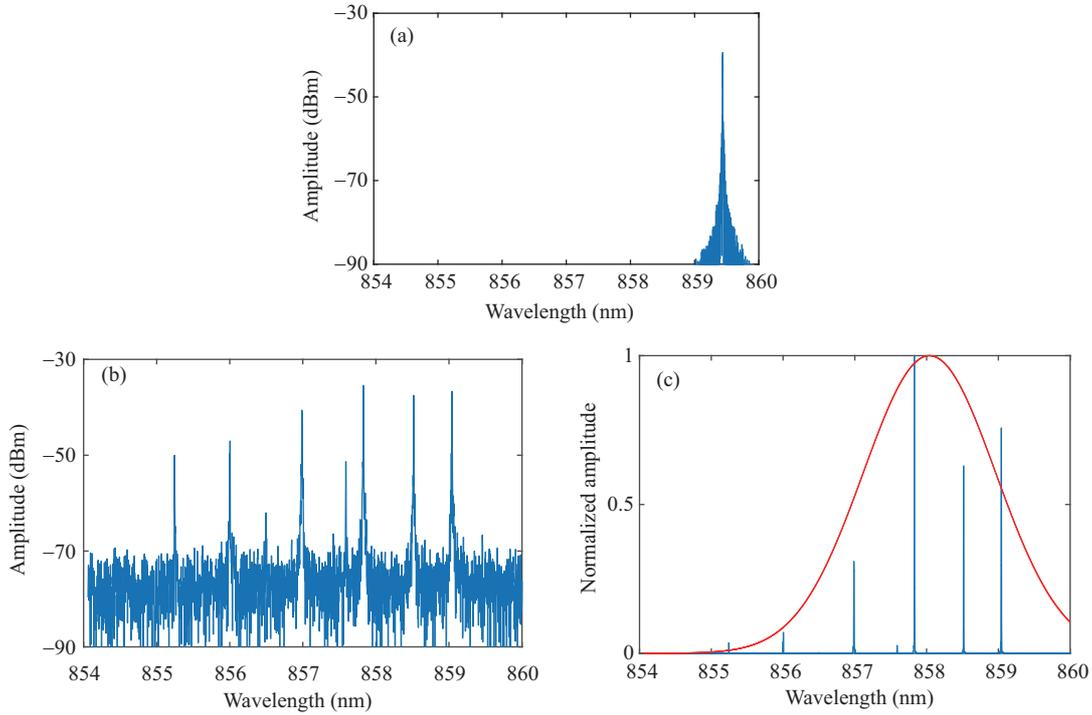
**Figure 3** (Color online) Optical spectrum of (a) VISTAS original, (b) VISTAS with our proposed method, and normalized optical spectrum of (c) VISTAS with our proposed method.
