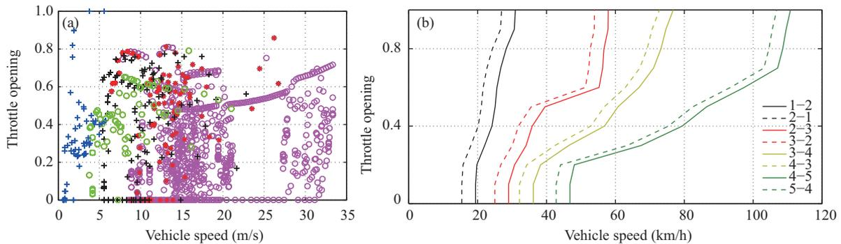
**Figure 1** (Color online) (a) Gear operational points of the three driving cycles and (b) the optimized DP-based gearshift schedule map.
