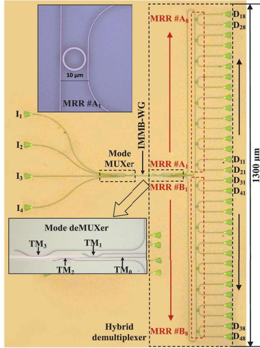
**Figure 6** (Color online) Fabricated hybrid MDM-WDM (de)multiplexer for TM polarization [89] ©Copyright 2018 IEEE.
