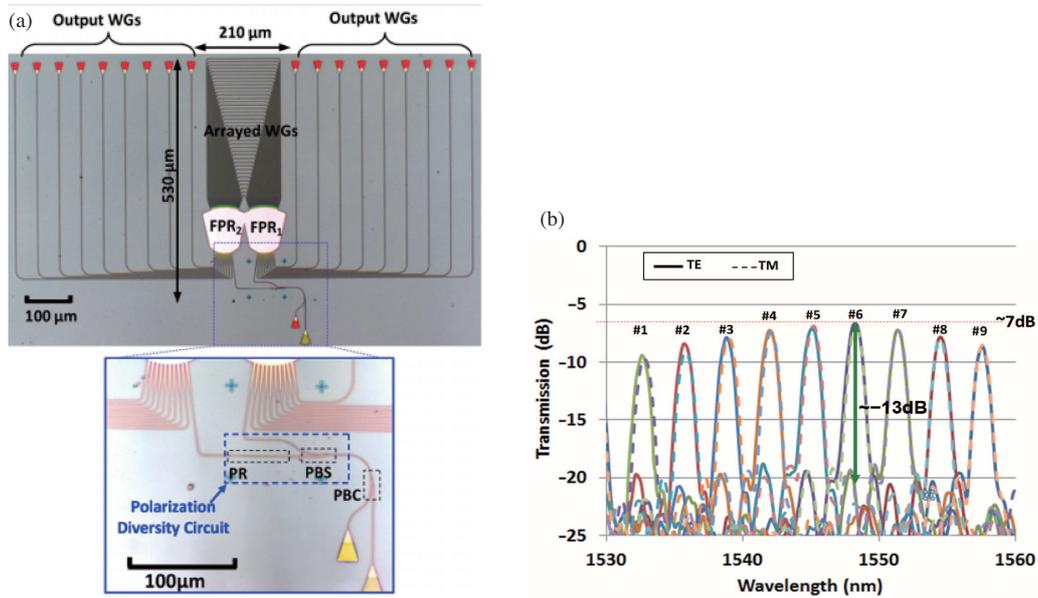
**Figure 2** (Color online) The hybrid WDM-PDM (de)multiplexer consisting of a bi-directional AWG and a polarization diversity circuit. (a) Microscopic image of the fabricated device; (b) measured spectral responses [69] ©Copyright 2015 OSA.
