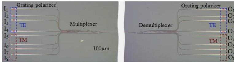
**Figure 9** (Color online) Fabricated PIC consisting of an improved 8-channel hybrid PDM-MDM (de)multiplexer [92] ©Copyright 2014 OSA.
