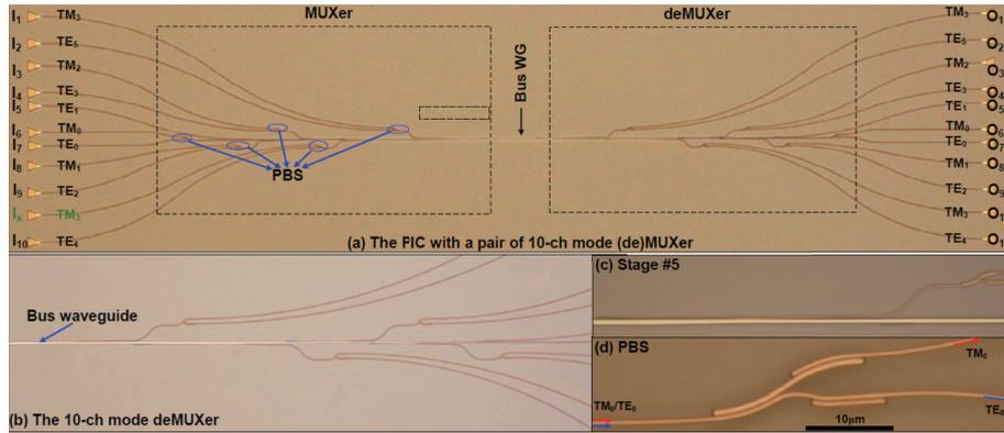
**Figure 10** (Color online) A 10-channel hybrid MDM-PDM (de)multiplexer based on dual-core adiabatic tapers waveguides with dual polarizations [95] ©Copyright 2017 Wiley.
