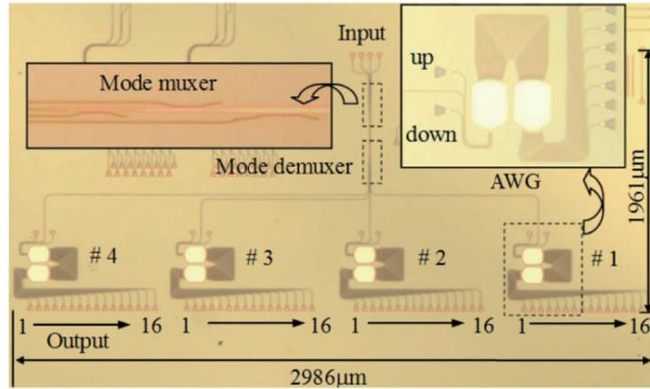
**Figure 4** (Color online) Fabricated 64-channel hybrid MDM-WDM (de)multiplexer consisting of a four-channel mode (de)multiplexer and four 16-channel AWG (de)multiplexers [83] ©Copyright 2014 OSA.
