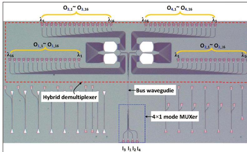
**Figure 5** (Color online) Fabricated 64-channel hybrid MDM-WDM (de)multiplexer consisting of a four-channel mode (de)multiplexer and two bi-directional AWG (de)multiplexers with 16 wavelength-channels [84] ©Copyright 2015 Wiley.
