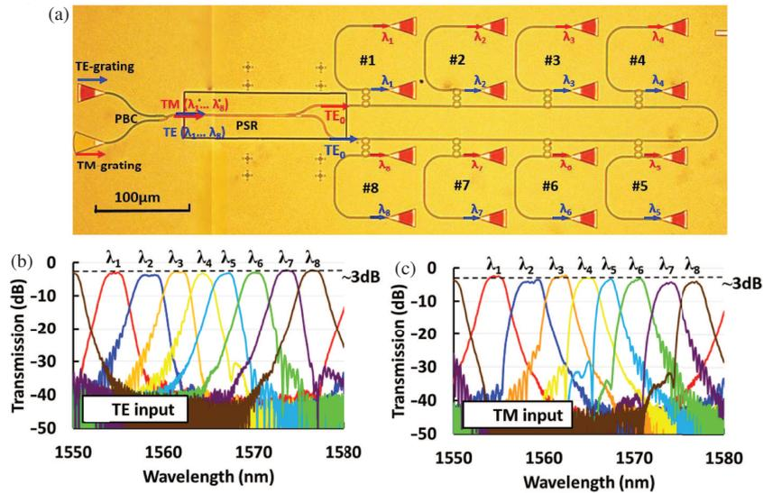
**Figure 3** (Color online) A 16-channel hybrid PDM-WDM (de)multiplexer. (a) Microscopic image. Measured spectral responses for all the channels of (b) TE- and (c) TM-polarizations [70] ©Copyright 2018 IEEE.
