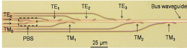
**Figure 8** (Color online) 8-channel hybrid PDM-MDM (de)multiplexer [91] ©Copyright 2014 Wiley.
