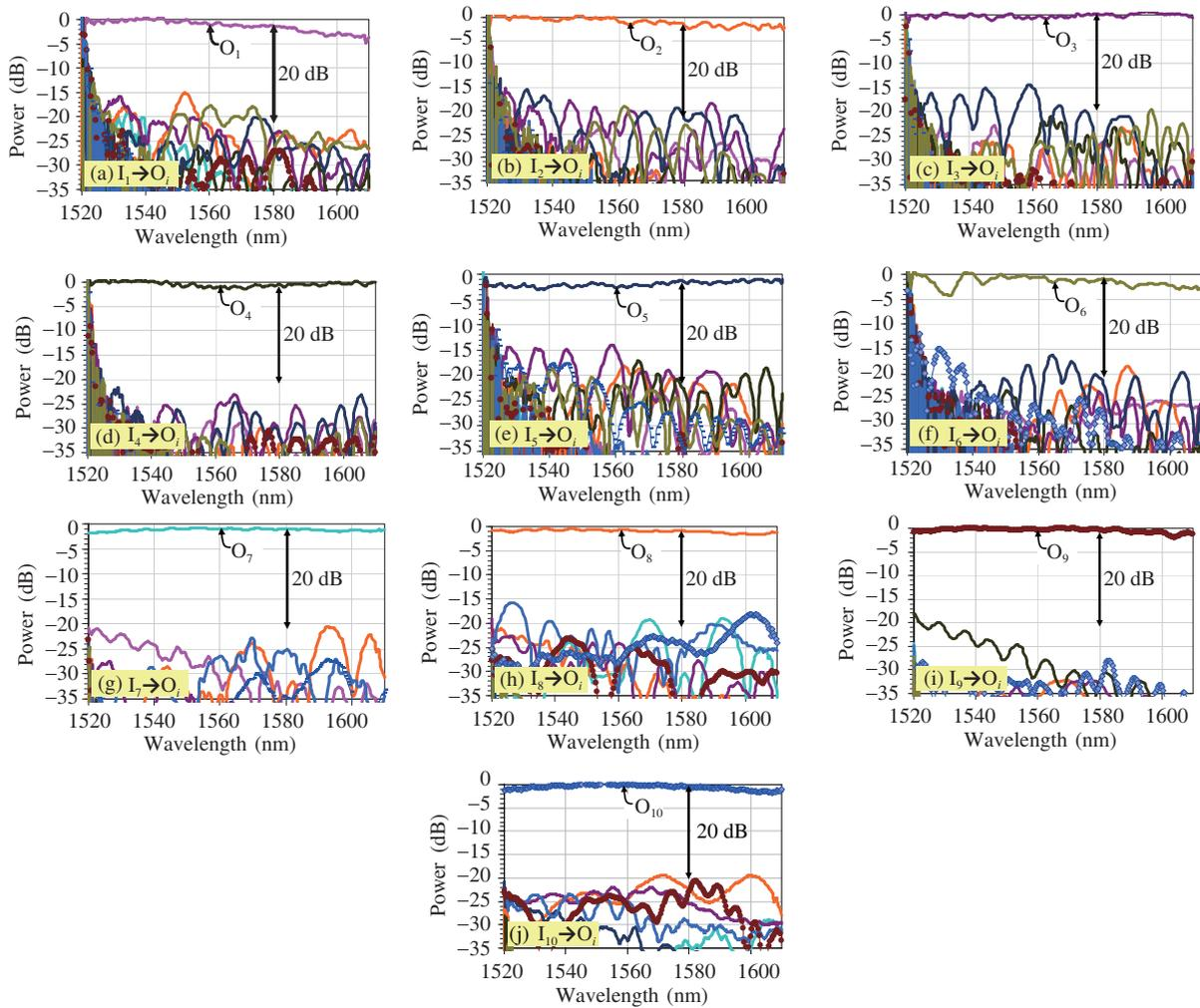
**Figure 11** (Color online) Measured transmissions at the then output ports ( $O_1 \sim O_{10}$ ) of the 10-channel hybrid MDM-PDM (de)multiplexer when light is launched from port (a)  $I_1$ , (b)  $I_2$ , (c)  $I_3$ , (d)  $I_4$ , (e)  $I_5$ , (f)  $I_6$ , (g)  $I_7$ , (h)  $I_8$ , (i)  $I_9$ , (j)  $I_{10}$  of the mode multiplexer, respectively [95] ©Copyright 2017 Wiley.
