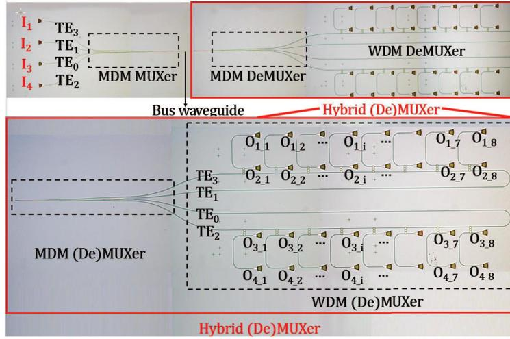
**Figure 7** (Color online) Fabricated hybrid MDM-WDM (de)multiplexer for TE polarization [82] ©Copyright 2018 OSA.
