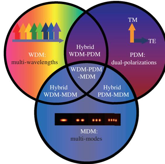
**Figure 1** (Color online) Hybrid (de)multiplexing technologies combining more than one techniques.
