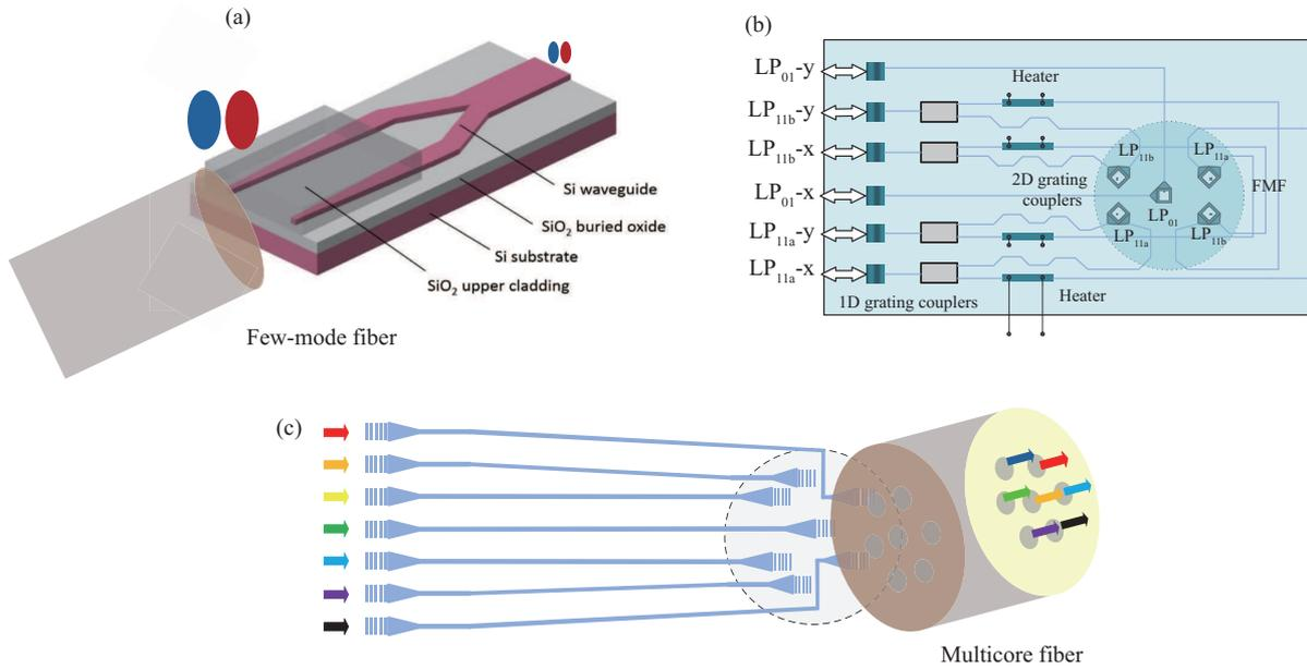
**Figure 2** (Color online) (a) Schematic structures of mode converter for fiber-chip coupling [21]; (b) mode MUX for FMMF fibers [25]; (c) MCF fan-in/fan-out [31].
