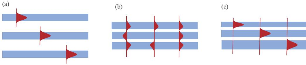
**Figure 5** (Color online) Guide modes supported in (a) waveguides far from each other, in (b) waveguides close to each other, and in (c) the proposed DPWA with optimized waveguide widths and separations.
