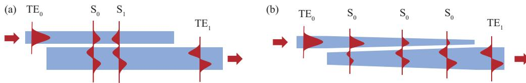
**Figure 3** (Color online) Schematic of the two supermodes propagating in (a) ADCs and (b) ACs.
