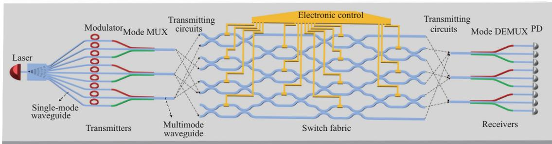
**Figure 9** (Color online) Schematic of an on-chip reconfigurable SDM system.
