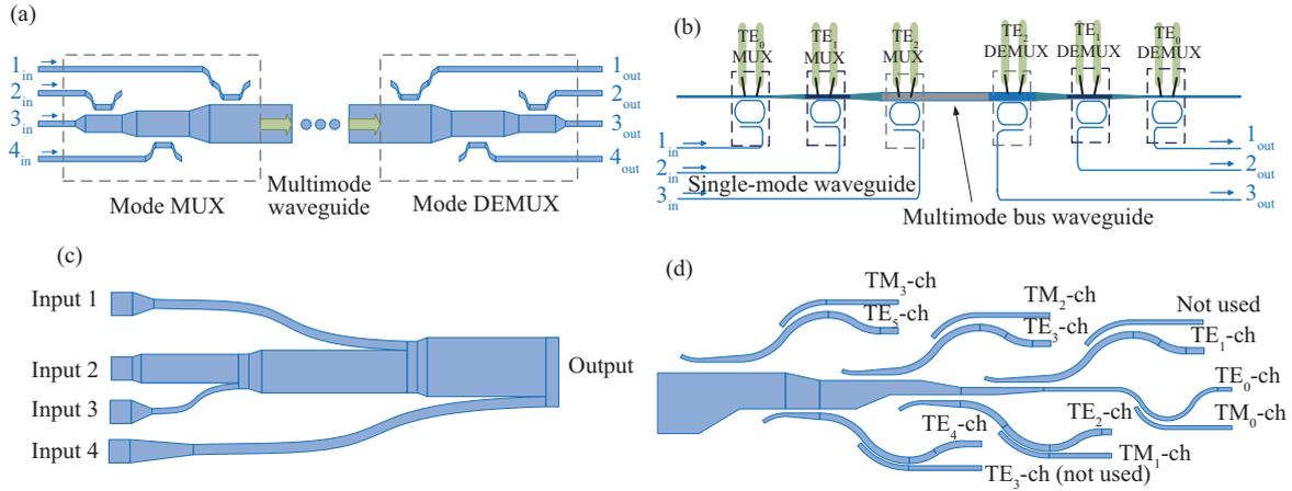
**Figure 4** (Color online) Schematics of multimode MUXs based on (a) ADCs [38], (b) MRRs [40], (c) Y-junctions [59], and (d) ACs [68].
