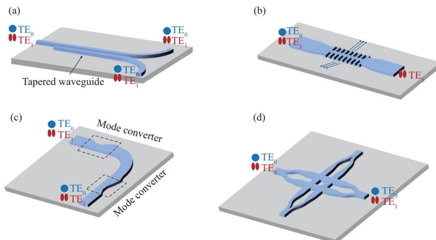
**Figure 6** (Color online) Three-dimensional structures of (a) multimode power splitter [81], (b) HOM pass filter [84], (c) multimode sharply bent waveguide [92], and (d) multimode waveguide crossing [107].
