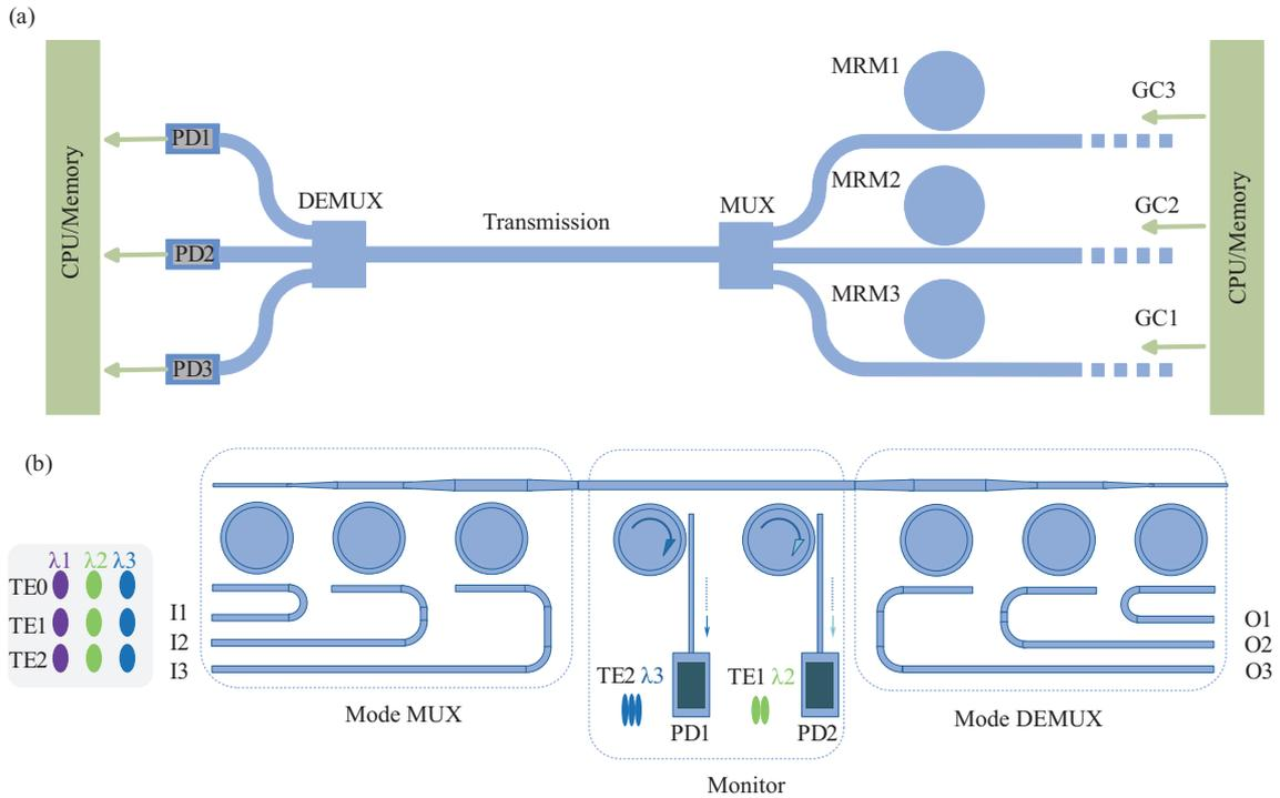
**Figure 8** (Color online) (a) Three-channel multimode PIC [145]; (b) non-invasive monitor for three-channel multimode PIC [157].
