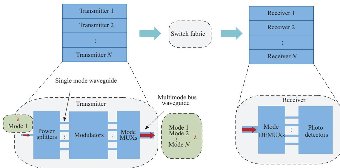
**Figure 1** (Color online) The schematic of an SDM system comprising  $N$  transmitters, a switch fabric, and  $N$  receivers. All the mode channels involved in the SDM system share the same wavelength.
