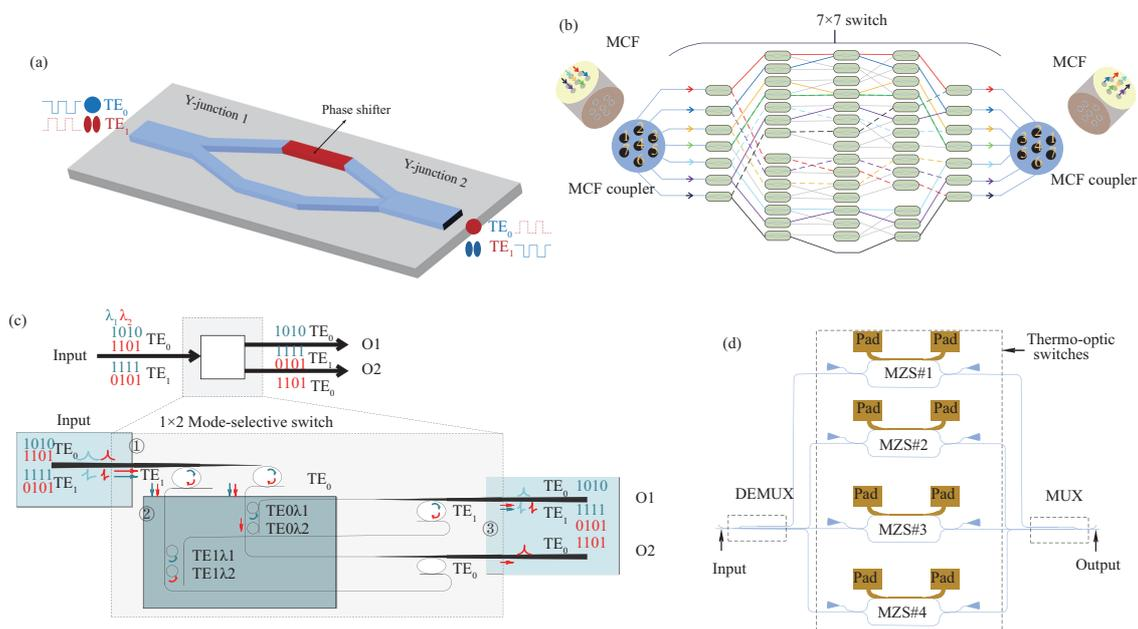
**Figure 7** (Color online) Schematic views of (a) dual-channel 1×1 mode-selective switch [119], (b) 1×1 mode-selective switch for seven-core fiber [121], (c) WDM-SDM 1×2 switch [123], and (d) four-channel reconfigurable add-drop multiplexer (ROADM) for multimode SDM [130].
