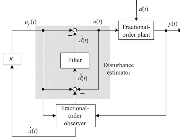
**Figure 1** The configuration of the FO control system.
