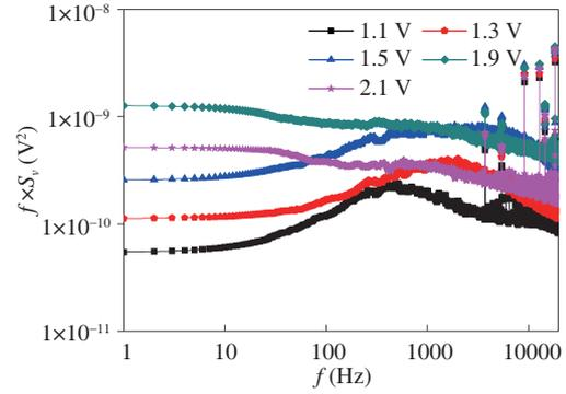
**Figure 1** (Color online) The normalized noise power spectrum density under different bias.
