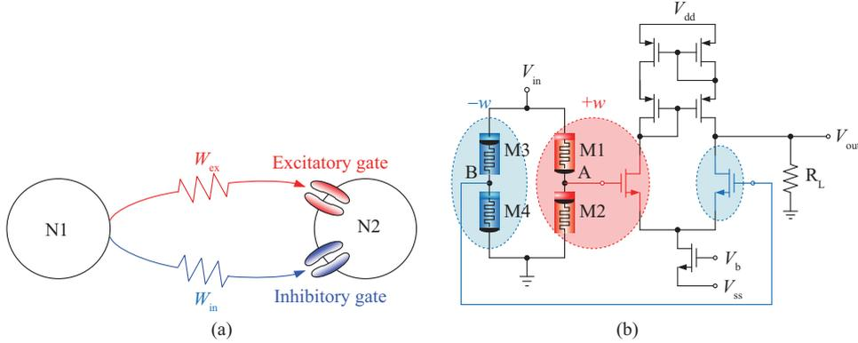
**Figure 1** (Color online) An architectural comparison between biological neuron and memristor bridge synapse-based artificial neuron. (a) Biological neuron; (b) memristor bridge synapse-based artificial neuron.
