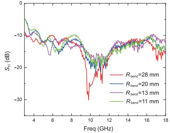
**Figure 8** (Color online) Measured reflection coefficient of the UWB RMA with O-slot when attached on cylinders of different curvature radius.
