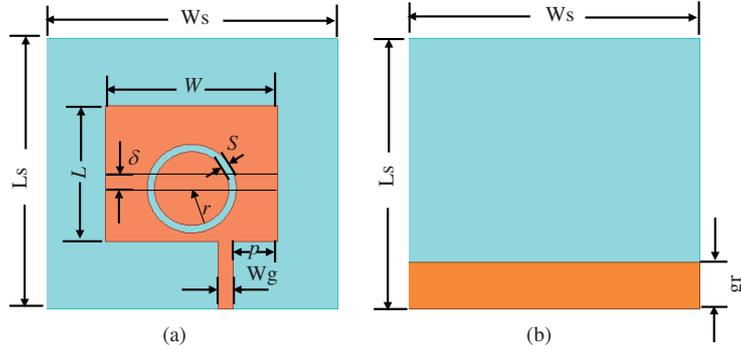
**Figure 1** (Color online) (a) Top view and (b) bottom view of the geometric layout of the O-slot UWB antenna.
