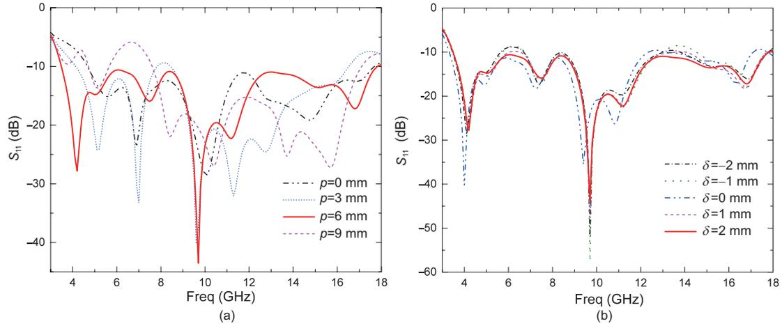
**Figure 4** (Color online) The simulated reflection coefficient of O-slot inserted UWB RMA with different (a) feed position,  $p$ , and (b) deviation distance of the O-slot,  $\delta$ . The other parameters of antenna are fixed with the parameters shown in Table 1.
