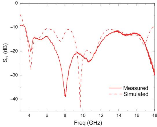
**Figure 7** (Color online) Simulated (dashed) and measured (solid)  $S_{11}$  parameters of the UWB RMA with O-slot at the frequencies ranging from 3 to 18 GHz
