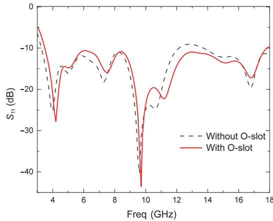
**Figure 3** (Color online) Simulated frequency response of the UWB RMA with/without O-slot.
