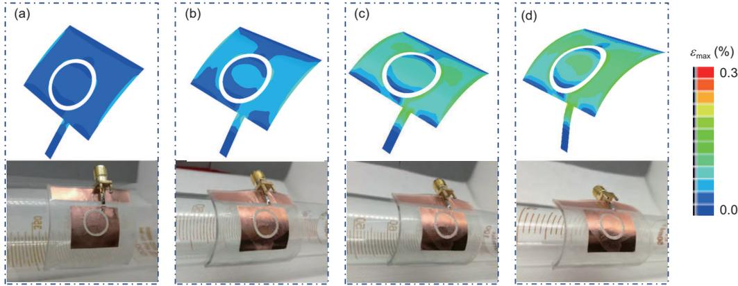
**Figure 6** (Color online) FEA results of the strain distribution on Cu layer and the corresponding optical images of the antenna with O-slot when attached on cylinders with different curvature radius. (a)  $R_{\text{bend}} = 28$  mm; (b)  $R_{\text{bend}} = 20$  mm; (c)  $R_{\text{bend}} = 13$  mm; (d)  $R_{\text{bend}} = 11$  mm.
