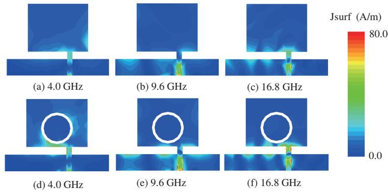
**Figure 2** (Color online) Simulation results of surface current distributions on the radiator of UWB RMA at three representative frequencies. (a)–(c) UWB RMA without O-slot; (d)–(f) UWB RMA with O-slot.
