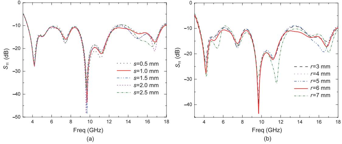
**Figure 5** (Color online) The simulated reflection coefficient of O-slot inserted UWB RMA with (a) different width of O-slot,  $s$ , and (b) different radius of O-slot,  $r$ . The other parameters of antenna are fixed with the parameters shown in Table 1.
