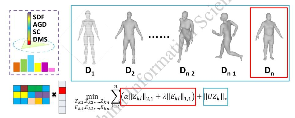
To better find the consistent expression of each class and the global common feature structure, we introduce the low rank constraints. And to achieve more compact feature representation, the rank of the global feature represent coefficients matrix should be low, as shown in the blue box.
