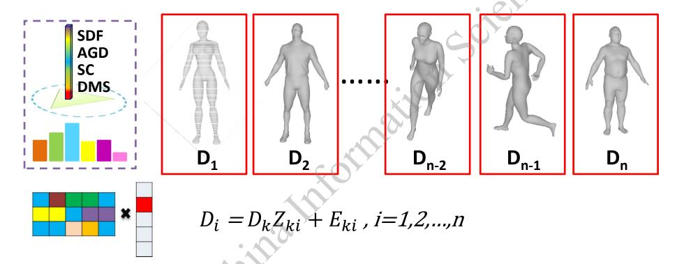
After pre-segmentation and features extraction processes, we convert the cosegmentation problem into feature clustering issues. Let  $D_i$  denotes patch features of model i, we first respectively adopt each single shape as dictionary to represent all the shapes in the same category with sparse constraint.
