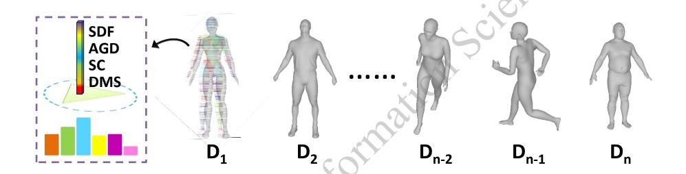
Input one 3D shape category, similar to Hu et al. [CGF 2012], we use normalized cuts algorithm to divide each shape into primitive patches for reducing computing complexity.
