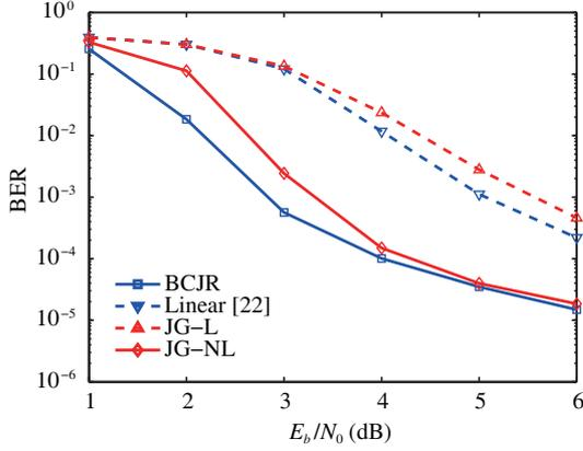
**Figure 2** (Color online) BER performance of the proposed JG-based turbo equalizers for BPSK signal.
