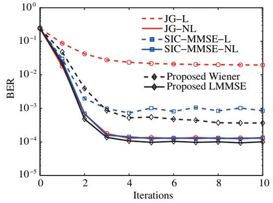
**Figure 5** (Color online) Convergence behavior for the proposed algorithms for BPSK signal.
