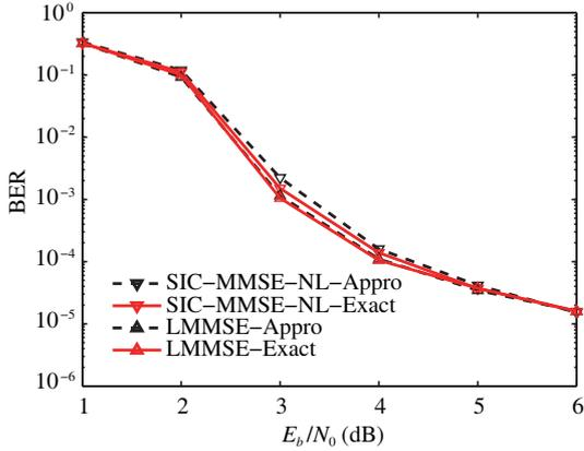
**Figure 6** (Color online) Performance comparisons by using the approximation in (39) and (40) for BPSK signal.
