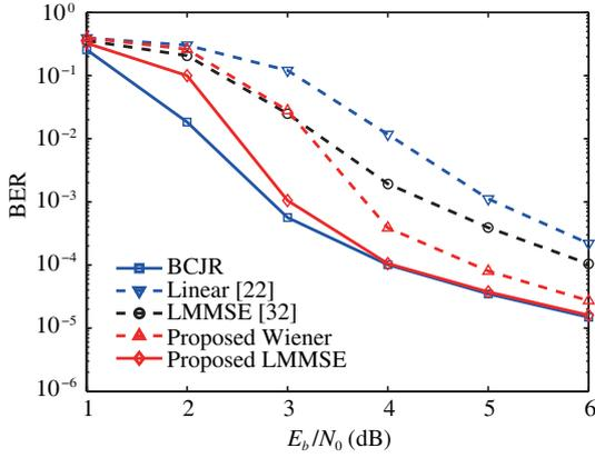
**Figure 4** (Color online) BER performance of the proposed LMMSE-based turbo equalizers for BPSK signal.
