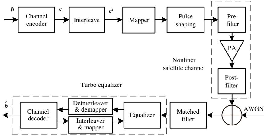
**Figure 1** Block diagram of the considered satellite communication system.
