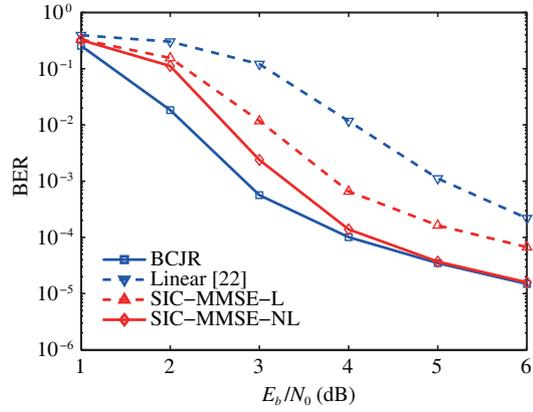
**Figure 3** (Color online) BER performance of the proposed SIC-MMSE-based turbo equalizers for BPSK signal.
