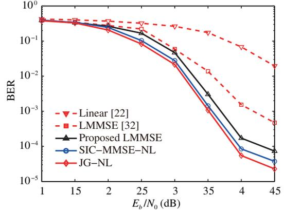
**Figure 7** (Color online) BER performance of the proposed algorithms for QPSK signal.
