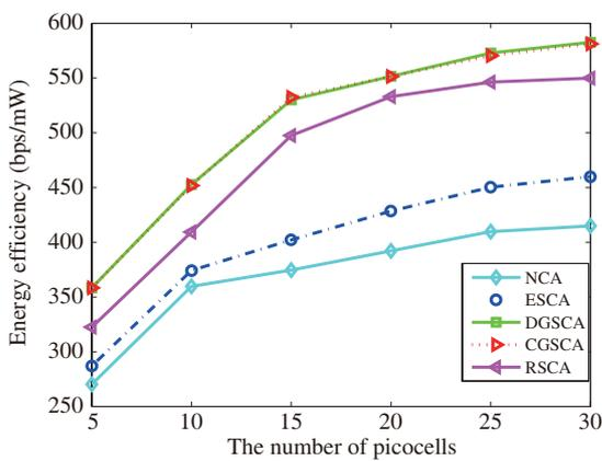
**Figure 5** (Color online) Variation in energy efficiency with an increasing number of picocells.
