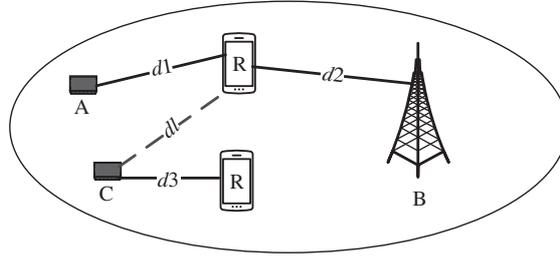
**Figure 2** Communication scenario of MTC network.
