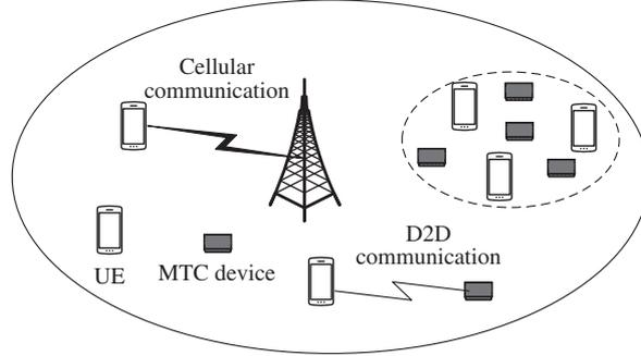
**Figure 1** Typical MTC system model.
