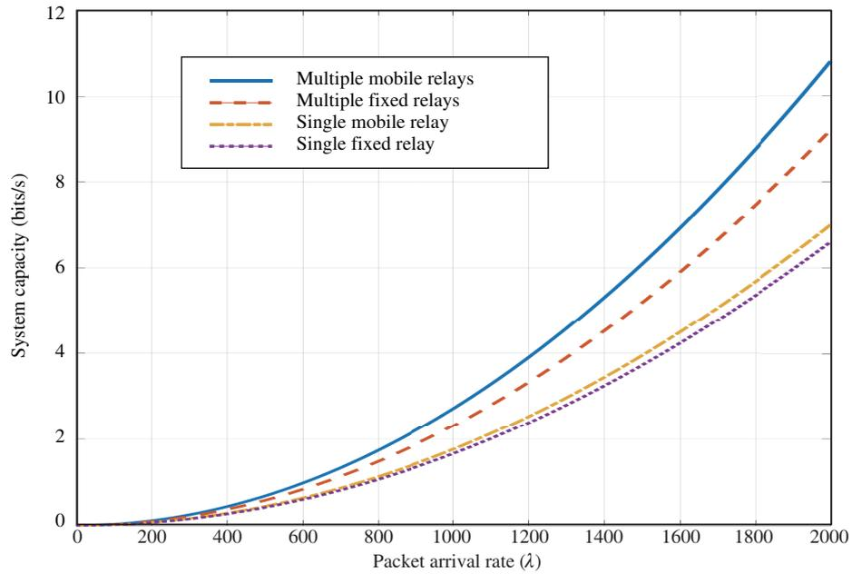
**Figure 9** (Color online) System capacity for increasing packet arrival rate.
