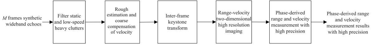
**Figure 2** Process flowchart of the phase-derived range and velocity measurement based on the synthetic wideband PD radar.
