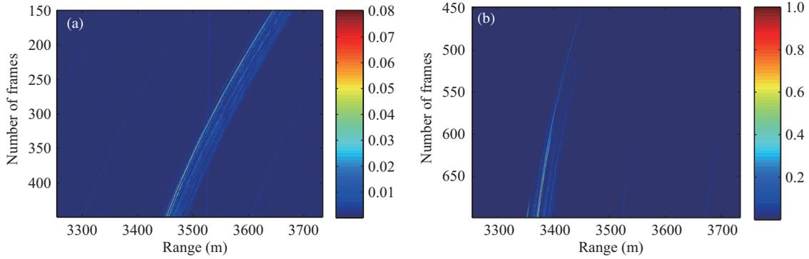
**Figure 8** One-dimensional HRRPs of the aircraft over time. (a) 150–500 frames; (b) 500–700 frames.
