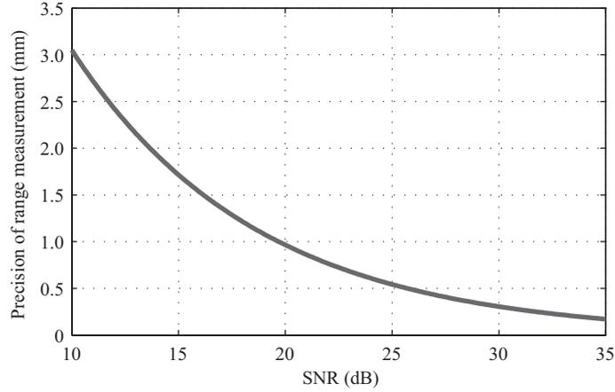
**Figure 1** Precision of the phase-derived range measurement at different SNRs.
