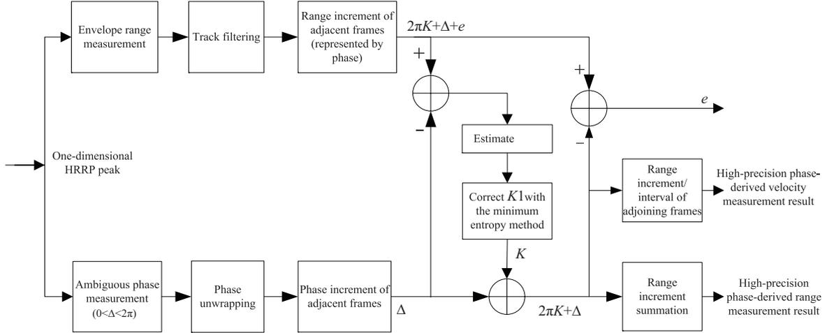
**Figure 3** Block diagram for the implementation of high-precision phase-derived range and velocity measurements.
