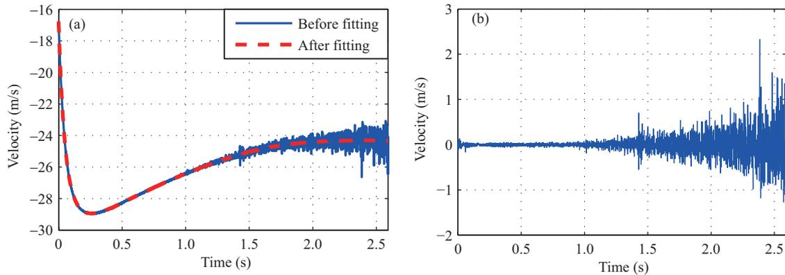
**Figure 7** Schematic diagram of the phase-derived velocity measurement results. (a) Phase-derived velocity measurement result; (b) phase-derived velocity measurement error.
