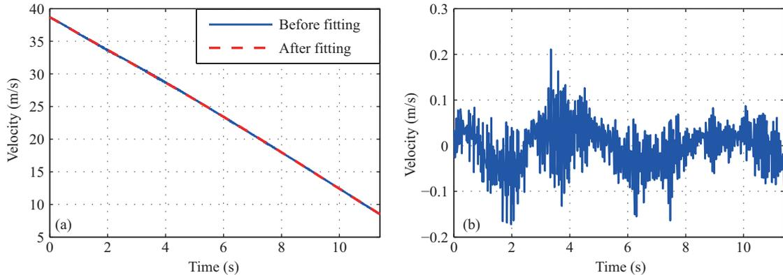
**Figure 10** Phase-derived velocity measurement results. (a) Phase-derived velocity measurement results; (b) phase-derived velocity measurement error.
