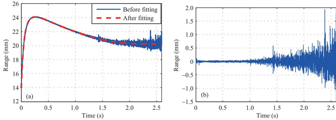
**Figure 6** Schematic diagram for the range increment measurement result and measurement error of adjacent frames. (a) Phase-derived range measurement result; (b) phase-derived range measurement error.
