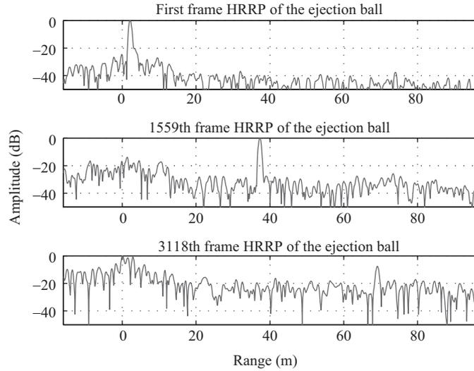
**Figure 4** One-dimensional HRRPs of the ejection ball at different moments.
