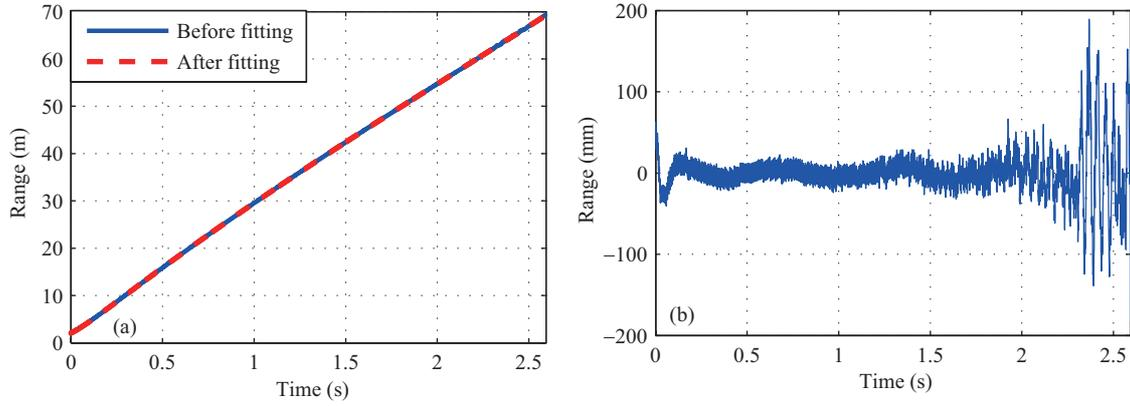
**Figure 5** Schematic diagram of the envelope range measurement result and error. (a) Envelope range measurement result; (b) envelope range measurement error.
