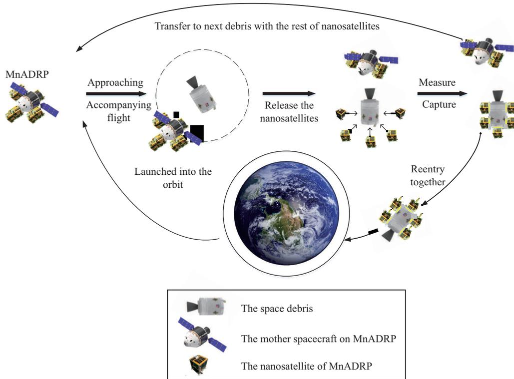
**Figure 1** Multiple space debris removal with MnADRP.
