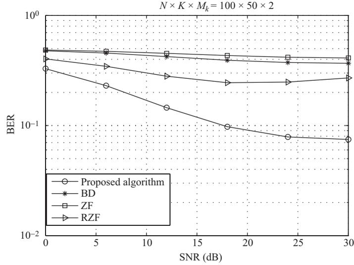
Figure 1 BER Comparison of different pre-coding algorithms.
