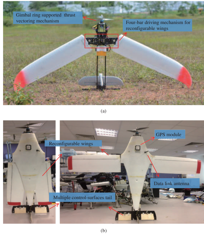
Figure 1 (Color online) Two prototypes for U-Lion. (a) U-Lion first prototype; (b) U-Lion current prototype.
