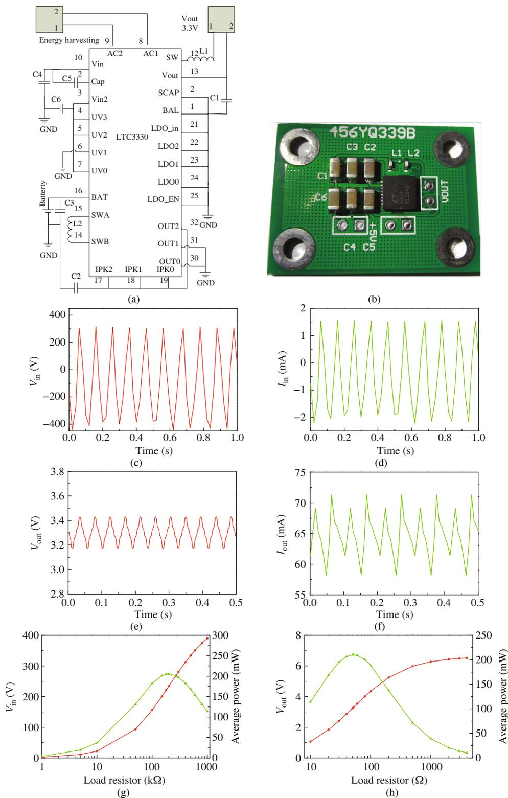
**Figure 1** (Color online) Optical photo of energy-harvesting system sample and test results. (a) The actual design circuit; (b) PCB sample of the system; (c) output voltage of the actual TENG; (d) output current of the actual TENG; (e) actual output voltage of power manager; (f) actual output current of power manager; (g) output voltage and average power of the TENG with different load resistors; (h) output voltage and average power of power manager system with different load resistors.
