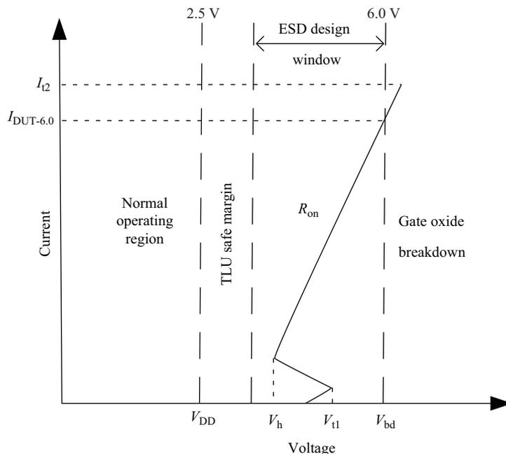
**Figure 1** ESD design window concerning the utilized process in this work.
