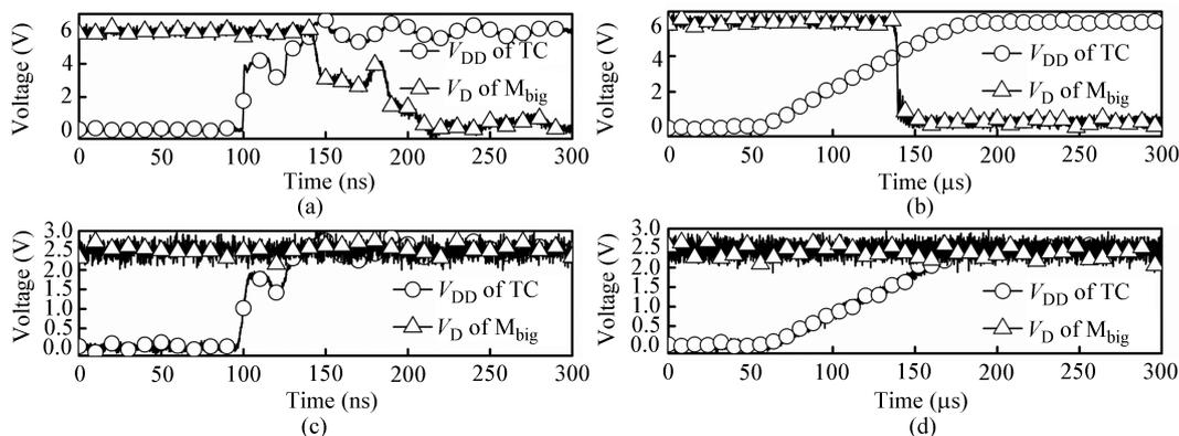
**Figure 7** Turn-on verification test results for the proposed circuit under different transient pulses on  $V_{DD}$  of TC with: (a) 5-ns rise-time and 6.0-V peak voltage, (b) 100- $\mu$ s rise-time and 6.0-V peak voltage, (c) 5-ns rise-time and 2.5-V peak voltage and (d) 100- $\mu$ s rise-time and 2.5-V peak voltage.
