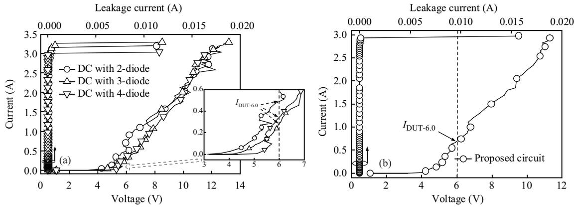
**Figure 6** TLP test results for: (a) DC circuits and (b) the proposed circuit.**Table 3** Summary of TLP test results for all investigated circuits
