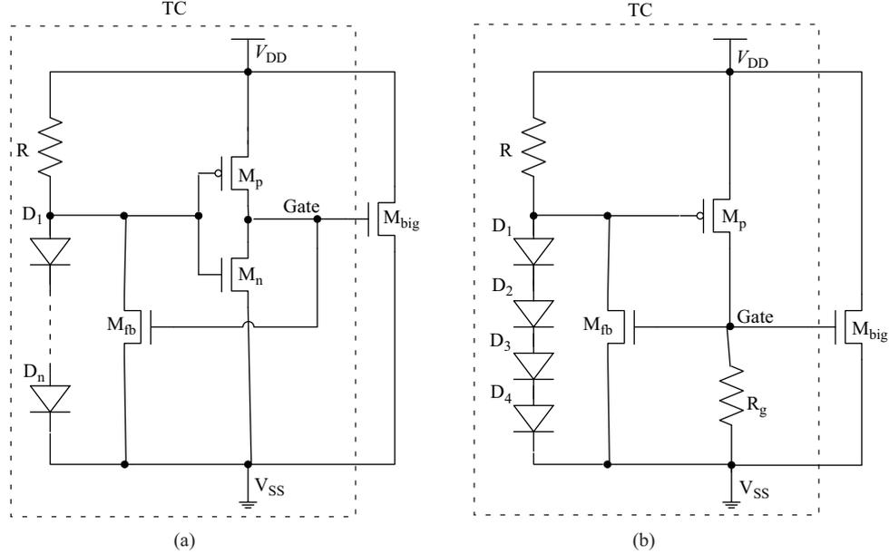
**Figure 2** (a) The traditional static-triggered power-rail ESD clamp circuit and (b) the proposed power-rail ESD clamp circuit.
