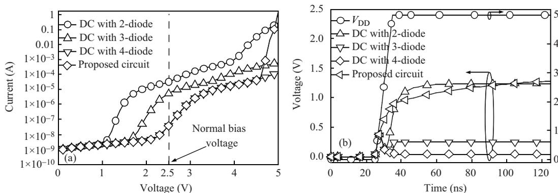
**Figure 3** (a) DC simulation results for all investigated circuits and (b) ESD-like transient simulation results for all investigated circuits.
