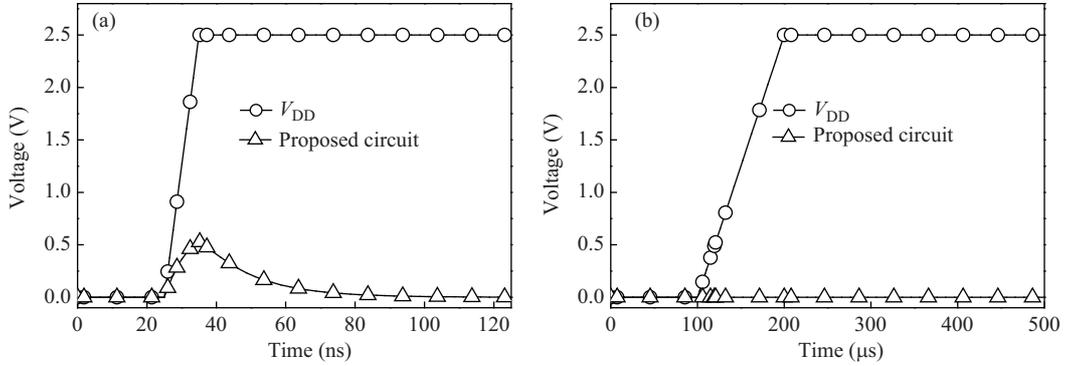
**Figure 4** Power-up simulation results for the proposed circuit (a) under a fast power-up pulse with a rise-time of 10 ns and (b) under a normal power-up pulse with a rise-time of 100  $\mu$ s.
