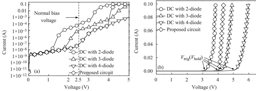
**Figure 5** DC test results for all investigated circuits: (a) F-V test results and (b) F-I test results.
