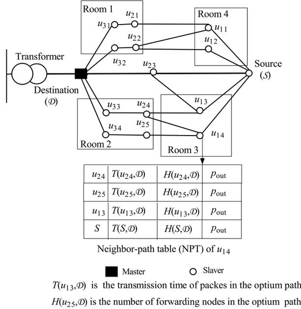
**Figure 3** A typical in-home PLC network topology.
