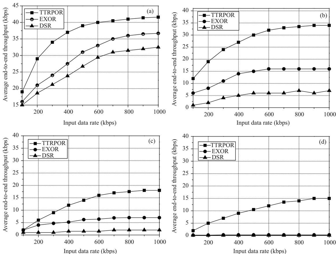
**Figure 7** End-to-end throughputs with different proportions nodes dynamically turned off. (a) All nodes working; (b) one-third of nodes turned off; (c) two-fifth of nodes turned off; (d) two-third nodes turned off.
