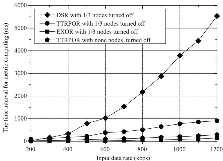
**Figure 8** Curves of time to compute the routing metric versus nodes dynamically turned off.
