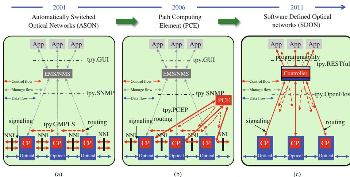
**Figure 5** (Color online) Various optical network control plane technologies. (a) GMPLS/ASON; (b) PCE; (c) Open-Flow/SDON.
