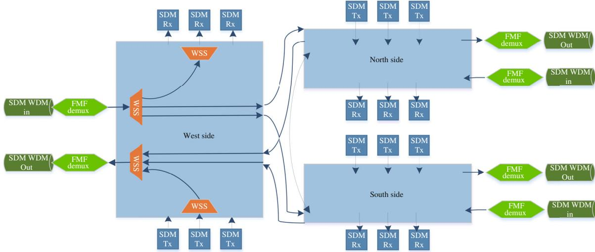
**Figure 4** (Color online) SDM switching node architecture.
