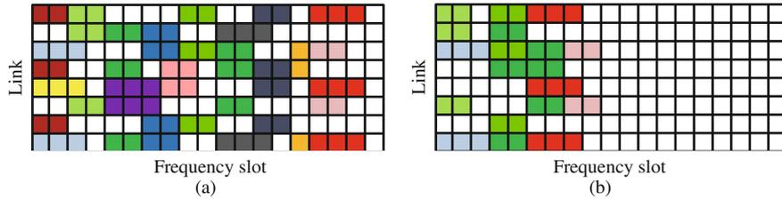
**Figure 7** (Color online) (a) Before spectrum defragmentation; (b) after spectrum defragmentation.
