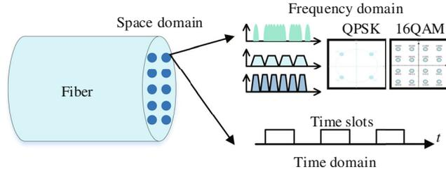
**Figure 1** (Color online) Illustration of multi-dimensional optical resources integration.
