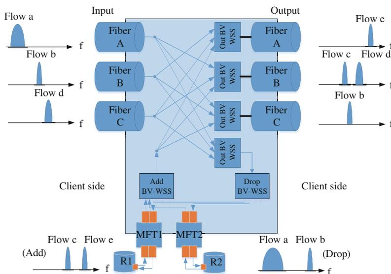
**Figure 3** (Color online) Elastic spectrum switching enabled by BV-WSS and MFT.
