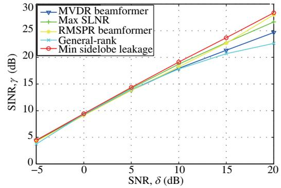
**Figure 5** (Color online) Output SINR versus the SNR.
