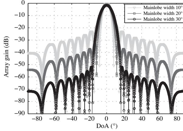
**Figure 1** The beam pattern of a ULA with various mainlobe widths.
