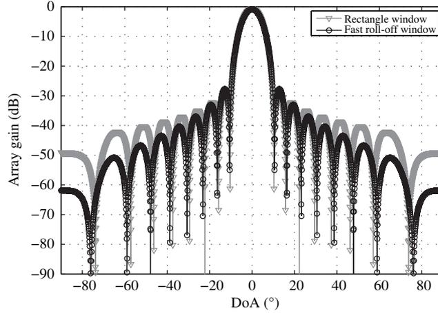
**Figure 3** A windowing beam pattern that has faster roll-off in the sidelobe.
