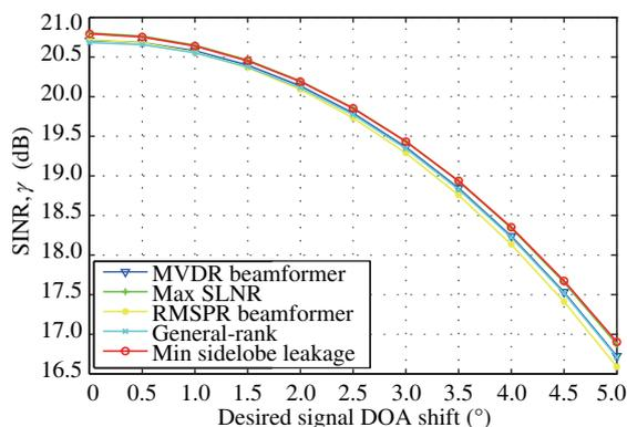
**Figure 6** (Color online) Output SINR versus the DOA mismatch of the desired signal.
