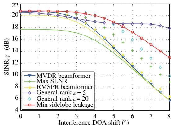
**Figure 7** (Color online) Output SINR versus the DOA mismatch of the interference.
