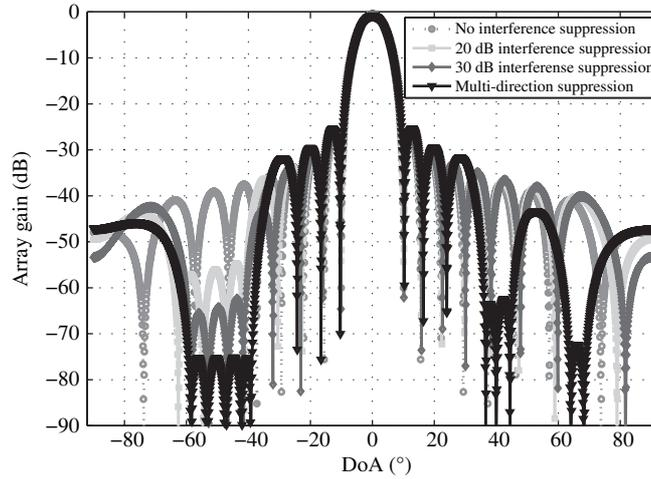
**Figure 2** The beam pattern of a ULA with various interference suppression levels.
