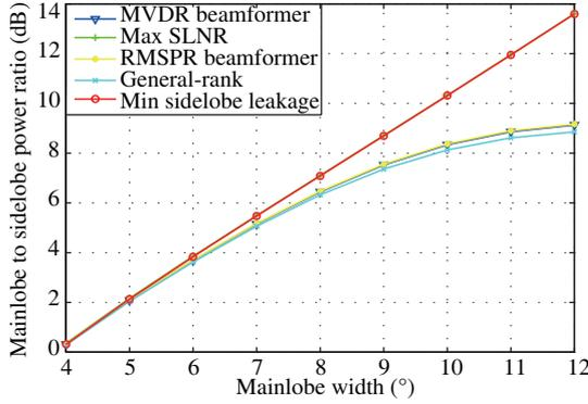
**Figure 4** (Color online) Mainlobe-to-sidelobe power ratio for various mainlobe widths.
