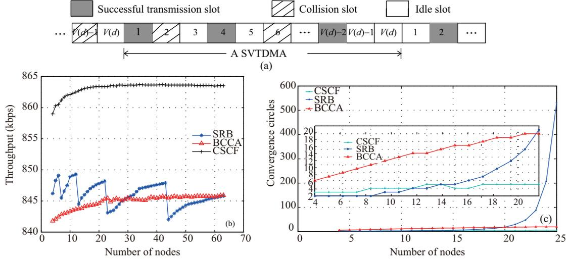
**Figure 1** (Color online) Example of SVTDMA and results of the experiment. (a) An example of SVTDMA; (b) convergence circle comparison; (c) the comparison of throughput between SRB-MAC, CSCF-MAC and BCCA.
