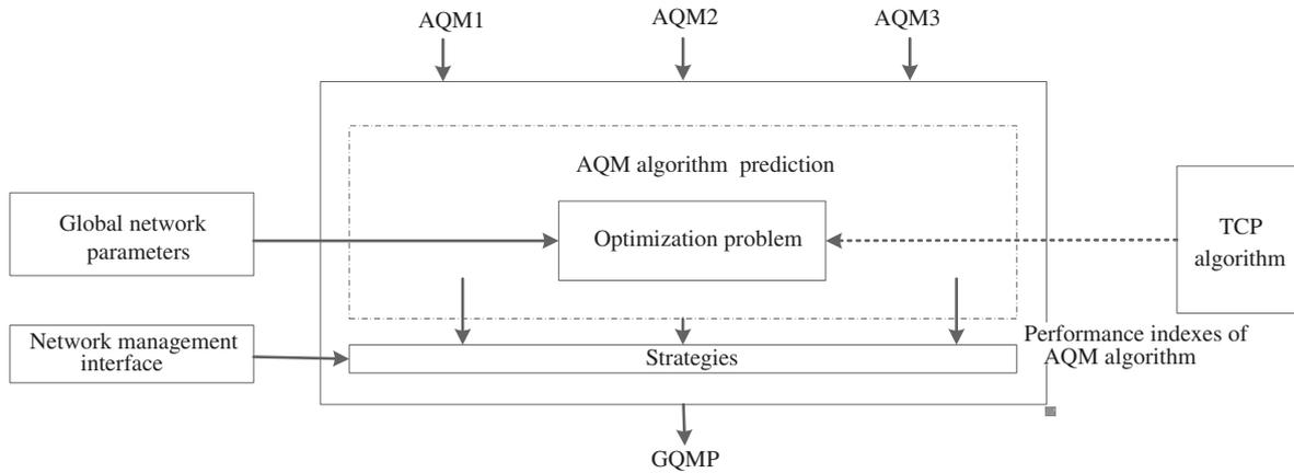
**Figure 8** Procedure of the network-layer centralized AQM selection scheme.
