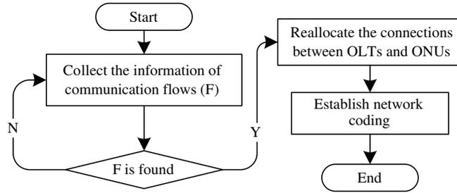
Figure 4 The flexible ONU matching process.
