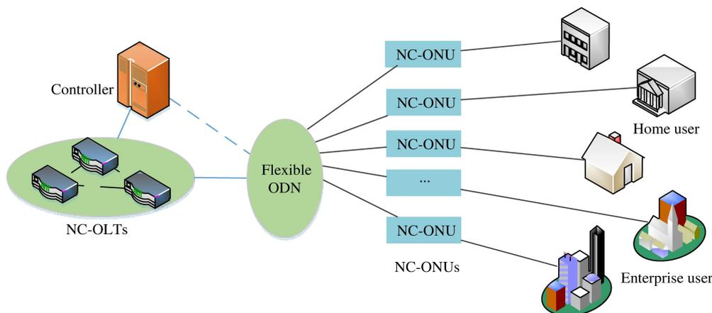
**Figure 3** (Color online) Operating scenario for the data-link-layer flexible coding scheme in the MODE-PON.
