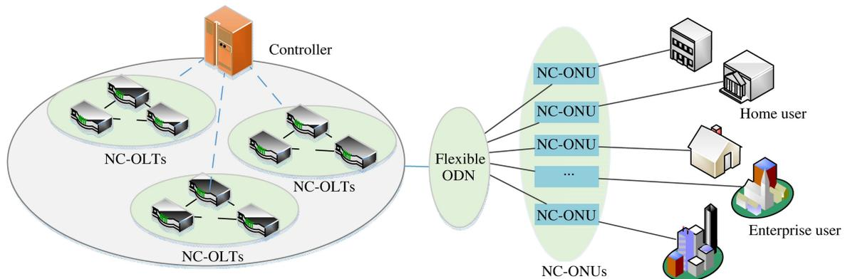
**Figure 2** (Color online) Multi-OLT-oriented efficient PON architecture.
