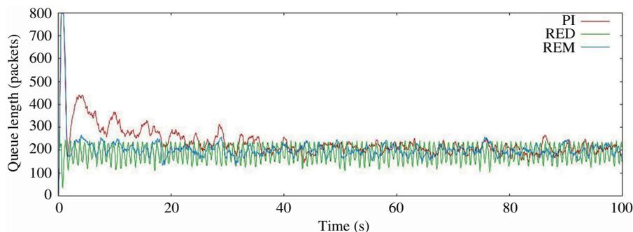
**Figure 10** Queue lengths of the RED, REM, and PI algorithms.
