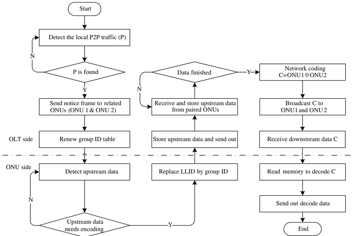
Figure 5 Flowchart of the network coding procedure in PON.
