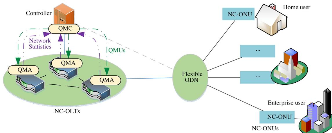
**Figure 6** (Color online) Operating scenario of the network-layer centralized AQM selection scheme in the MODE-PON.
