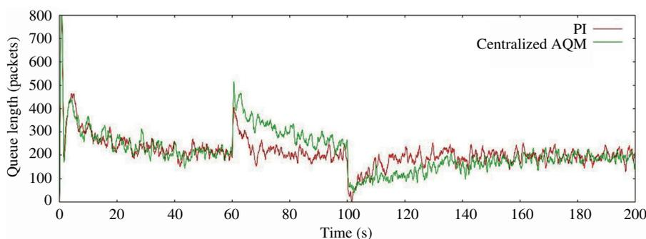
**Figure 11** Comparison of queue lengths of PI and PI with centralized AQM.
