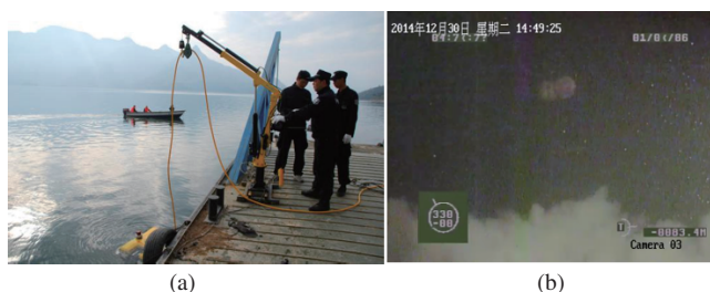
图 6 (网络版彩图) (a) ROV 从船边下放; (b) 根据 ROV 位置下放标志物 Figure 6 (Color online) (a) Drop ROV from shipside; (b) drop markers based on the location of ROV
